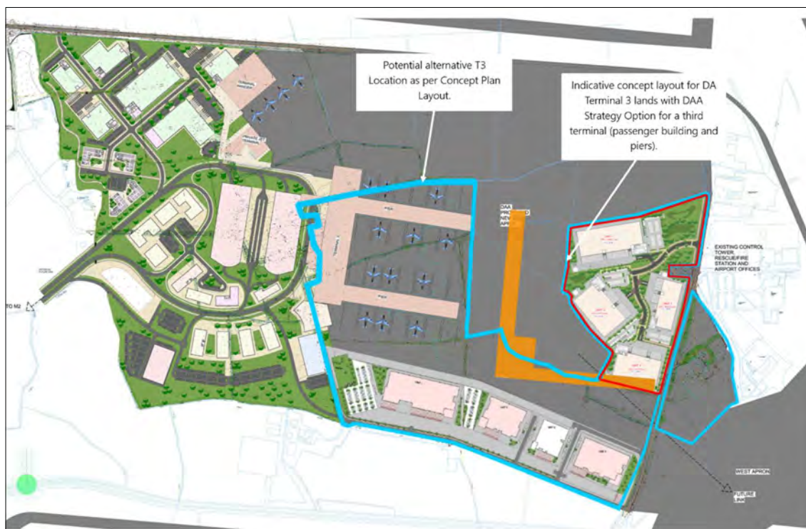
Figure 3.5: Indicative concept layout for DA Terminal 3 lands with DAA Strategy Option for a third terminal (passenger building and piers). Source: CWPA
