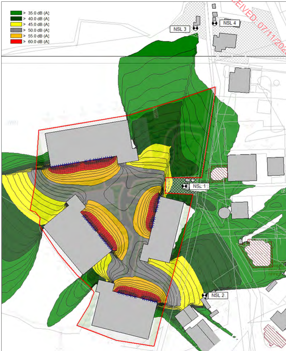
Figure 10.11: : L_{Day} noise map 4m above ground. Stated values are A-Weighted for the specific sound level.
